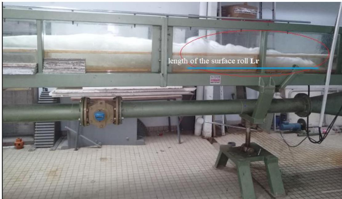
**Photograph 1.** the formation of the surface roll length for a hydraulic jump in a rectangular channel of a compound section with a rough bottom.
