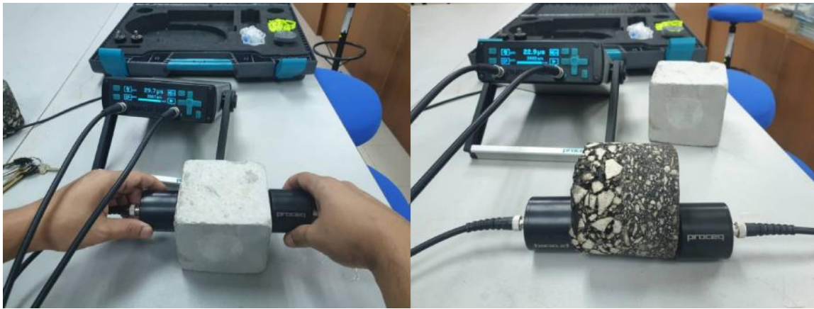
Fig.3. P-wave velocity measurement using the Pundit test.
