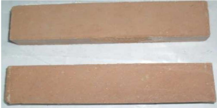
Fig.2 Prismatic brick based on mud from dredging
