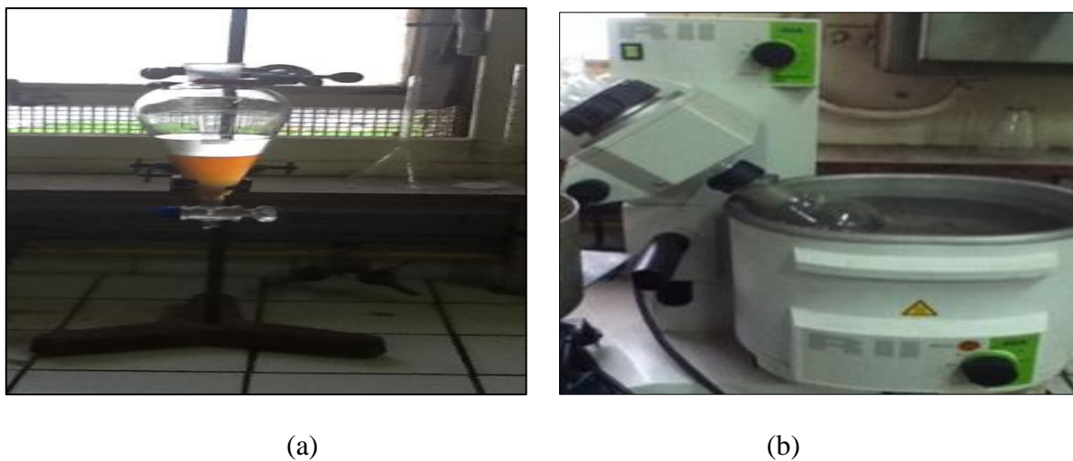
Fig.4. Purification of raw extracts: Liquid-liquid extraction (a) , Vacuum distillation (b)
