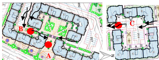
Fig. 6. Wind flow between buildings in winter
