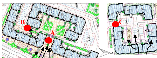
Fig.9. Wind flow between buildings in summer
