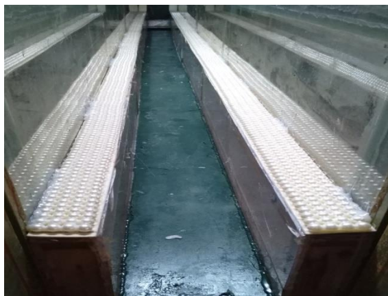
Photograph of a rough carpet carefully glued to the bed major of the rectangular channel of compound section Photograph of the four rough mats: \varepsilon=06 mm, \varepsilon=08 mm, \varepsilon=10 mm and \varepsilon=12 mm
