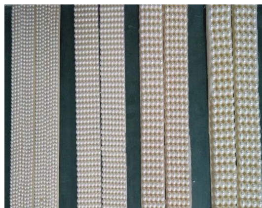
Photograph of a rough carpet carefully glued to the bed major of the rectangular channel of compound section Photograph of the four rough mats: \varepsilon=06 mm, \varepsilon=08 mm, \varepsilon=10 mm and \varepsilon=12 mm
