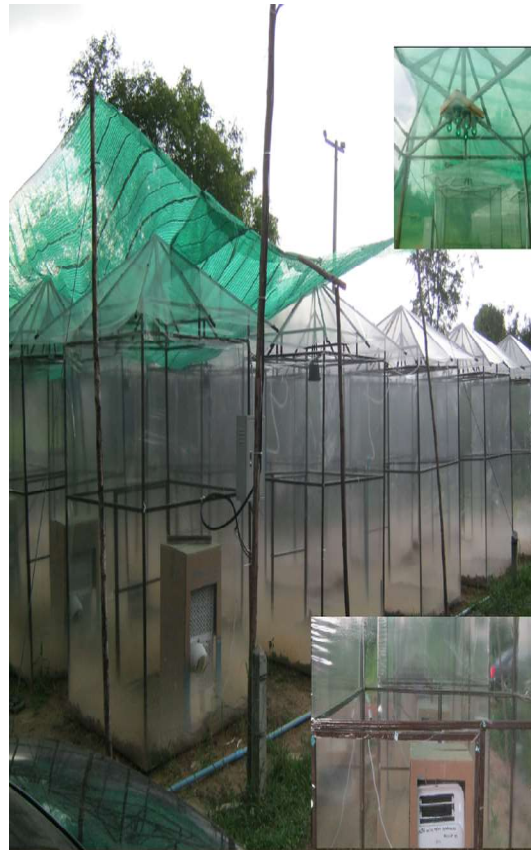
Fig.1. Square Open Top Chamber (OTC) for temperature controlling for field experiment
