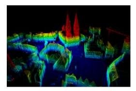
**Fig.1.** Object modeling using Lidar and SLAM(Nuechter, 2016)
