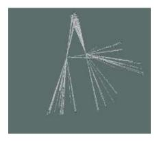
The first deformation is shown in Fig.5 in the bottom right corner. This deformation is caused by a smooth wall, where an algorithm detects a small number of interesting points and calculates the deformed space map. The second problem is in the top left corner. This error is caused by ray reflection in the mirror on the wall. The red line shows the calculated trace using Hector SLAM. Other examples of space mapping are shown in Fig.6 and Fig.7.
