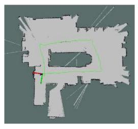
Fig.6. Example of closed path mapping (length 10m)
