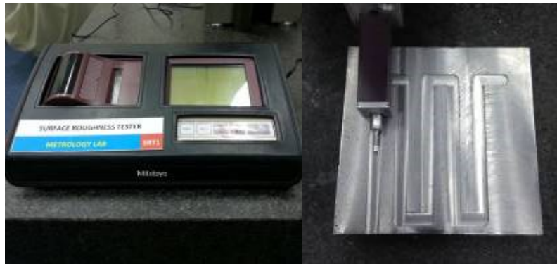
Fig.12. Surface roughness tests on machining profile
