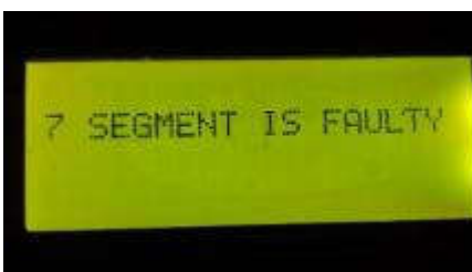
(a) Feedback for faulty 7segment display
