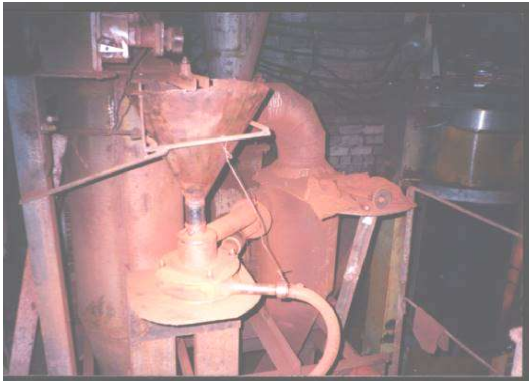
Fig.12. General view of a pilot-industrial sample of a vortex-acoustic dispersant
