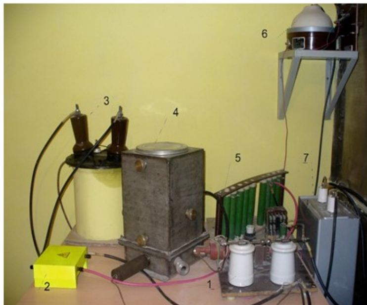
Fig.1. The device for high-voltage processing of bioorganic waste. 1 - air gap; 2 - voltage stabilizer; 3 - tension transformer; 4 - digit camera bioreactor; 5 - resistor block; 6 - high-voltage measuring instrument; 7 - condenser.
