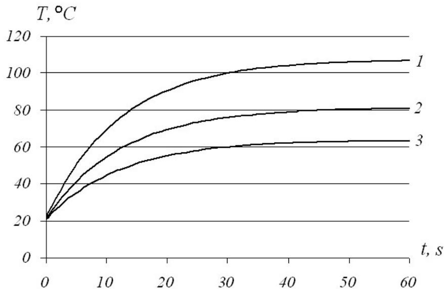
**Fig.4.** Time dependences of LED crystal temperature at different values of power emitted in it: 1 —  $p_1=1$  W; 2 —  $p_2=0,7$  W; 3 —  $p_3=0,5$  W.
