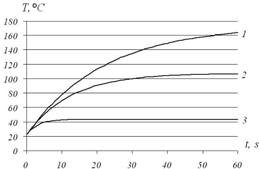
**Fig.5.** Time dependences of crystal temperature for various cooling methods: 1 - without additional cooling; 2 - cooling by a printed circuit board; 3 - cooling by the radiator.
