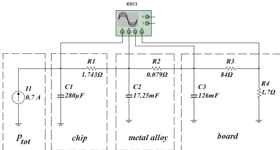
**Fig.3.** LED heat model in Multisim.
