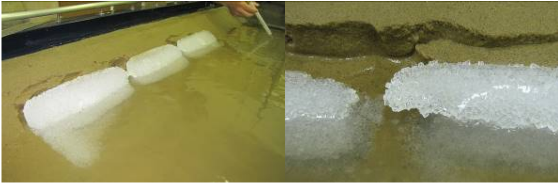
Fig.3. Influence of the flow on the underwater erosion of thawed material
