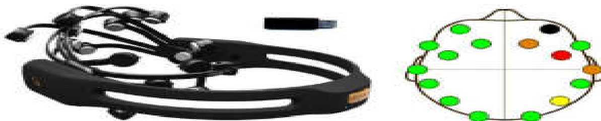
Fig.1. Emotiv EPOC neuroheadset and the locations of its 16 sensor [16]
