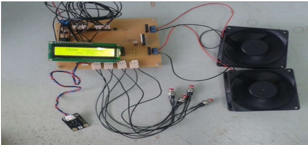
Fig.5. Circuit simulation of smart ventilation fan on PCB board
