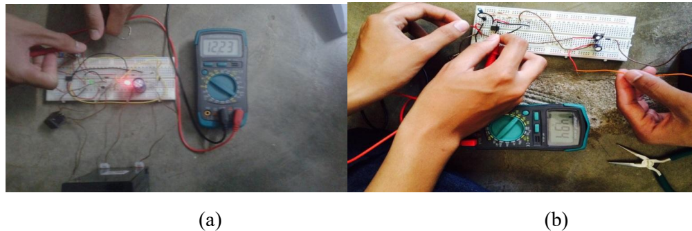
Fig.10. The measurement of voltage on the circuits (a) Output rechargeable battery (b) Output voltage regulator circuit
