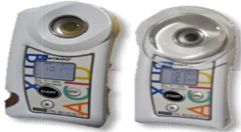
**Fig.4.** (Left) Refractometer shows the reading of Brix (Right) Refractometer shows the reading of Brix and acidity
