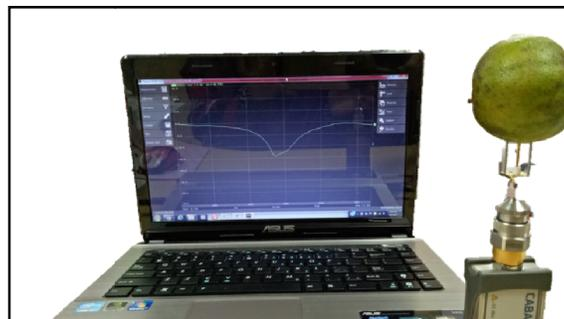
**Fig.3.**  $S_{11}$  is being measured using CABANR54
