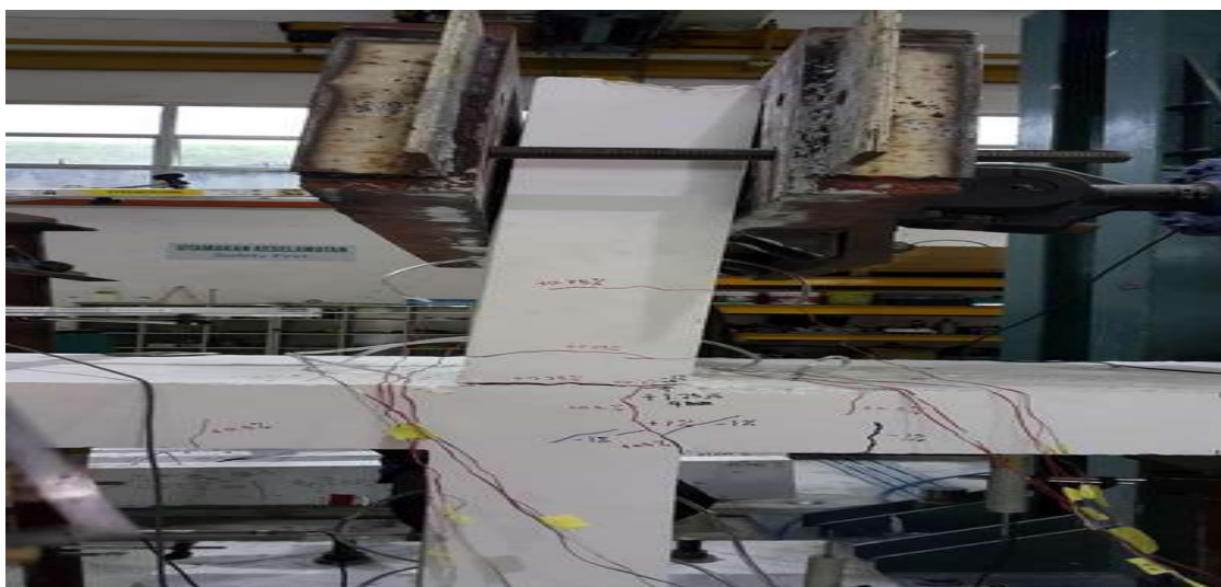
Fig.15. Cracks occurred at wall-slab joint
