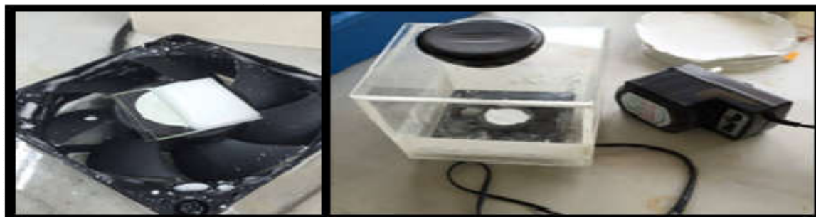
Fig.4. A homebuilt spin coater contained in PMMA box with a modified DC adapter
