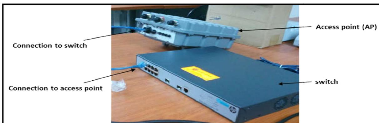
**Fig.4.** Equipment set up
