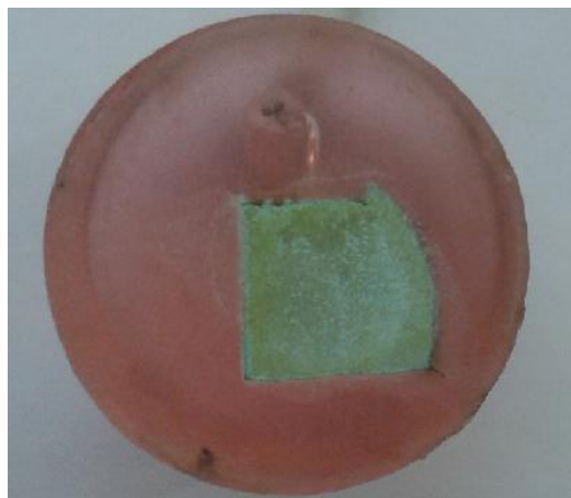
Fig.8. Formation of greenish colour of \text{CuCl}_2 on the sample
