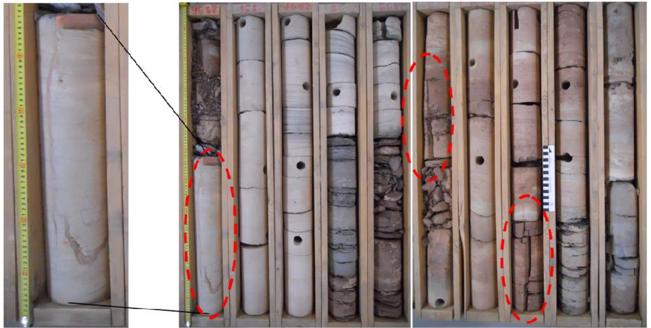
Fig.16. Photos showing reddish salt filled fracture in sandstone of top TAGS, from 2889 to 2894 m
