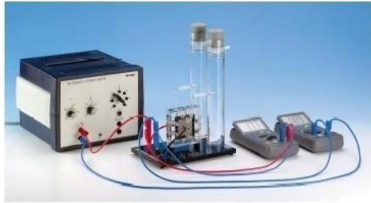
Fig.3. Production of hydrogen with an electrolyser supplied by a generator in the CDER laboratory
