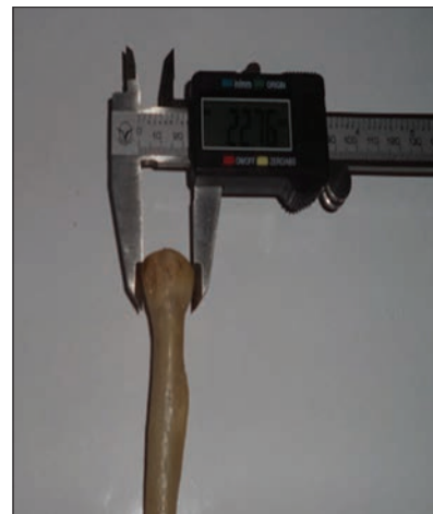
Plate 2: Measurement of maximum head diameter of the radius using a digital vernier caliper
