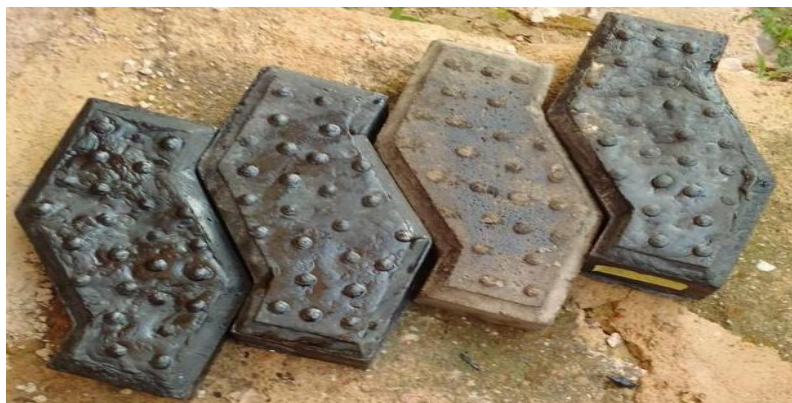
Plates 3a & 3b: Developed plastic pavement block composites
