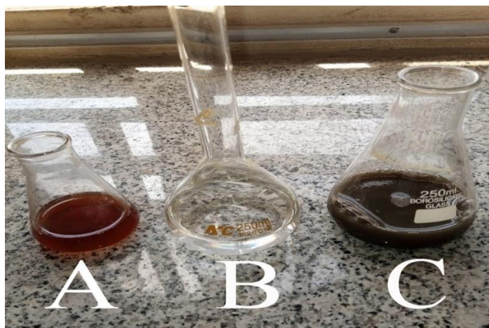
Plate 1: (a) Lantana camara aqueous leaves extract (b), silver nitrate solution (c), solution of silver nanoparticle
