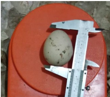
Photo 2: Length and width measurement with a vernier calliper
