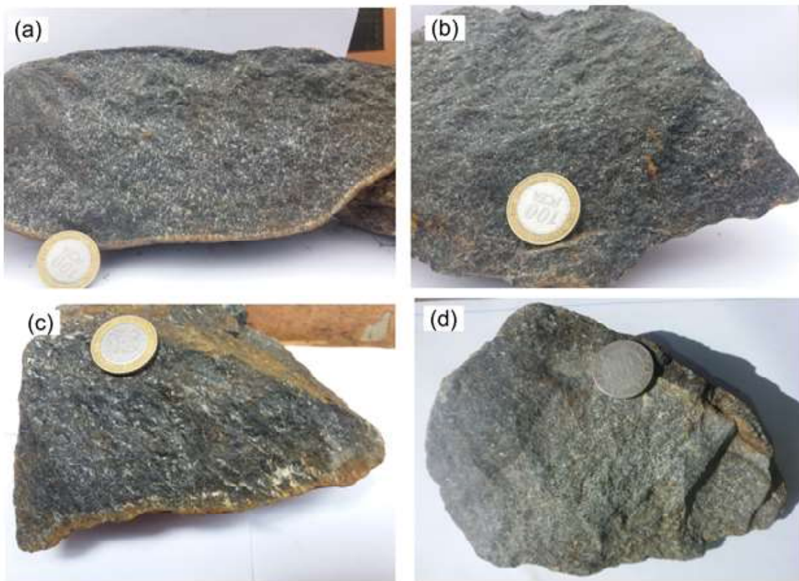
Fig. 6: (a) Amphibolite showing medium grain granular texture with minerals such as amphiboles (hornblende), quartz and accessory sulphide (b) Coarse grain amphibolite, pinkish in color with amphiboles, and quartz (c) Coarse grain amphibolite with schistosity define by preferred alignment of amphiboles minerals. (d) Garnet bearing amphibolites showing a medium to coarse-grained textures.
