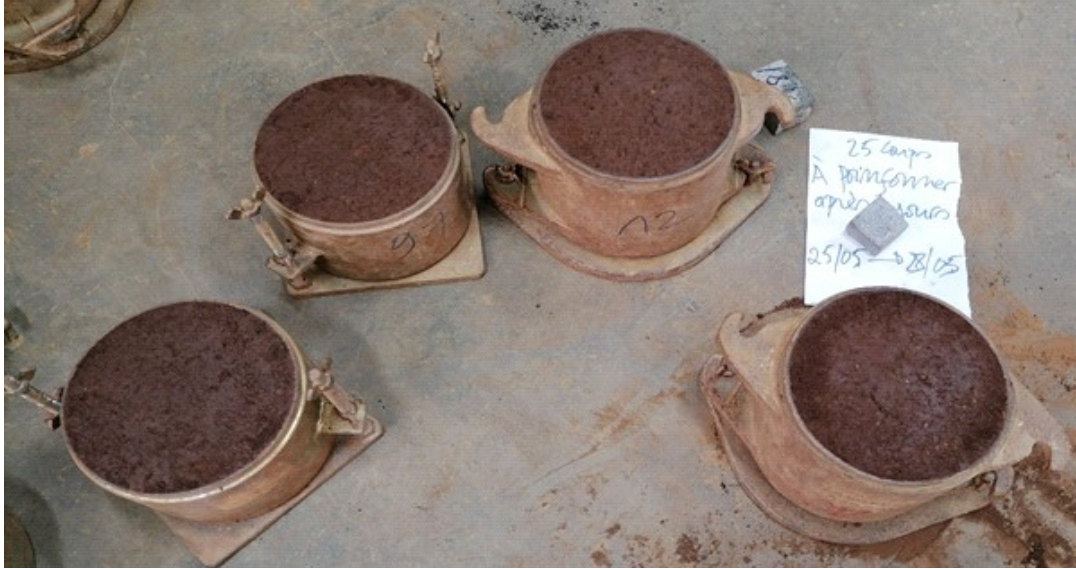
Figure 8: CBR evidence of soil treated with AggreBind/RoadMaster
