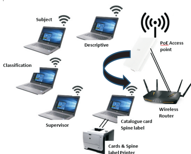
Figure 2. Systems Deployment Design
