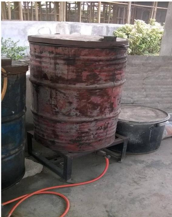
Plate 1: Fabricated Wet Steam Sterilizing Unit.
