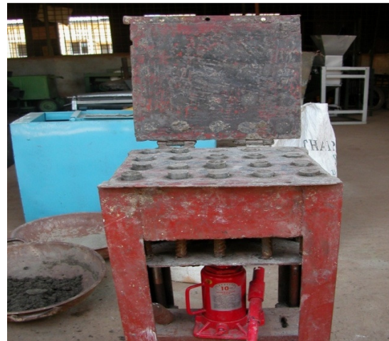
Fig 1: Fig 1: Briquette Moulding Machine Showing Ejection Pistons
