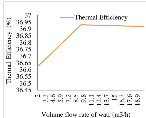
Fig. 8: Effect of variation of volume flow rate of water on thermal efficiency of gas turbine
