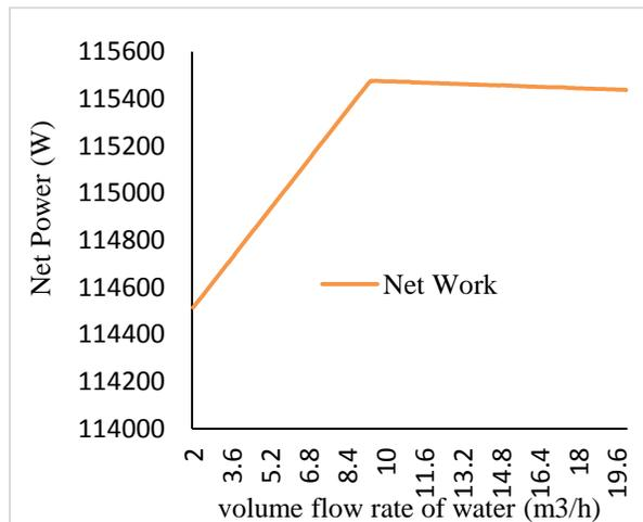
Fig. 9: Effect of variation of volume flow rate of water on net power of gas turbine
