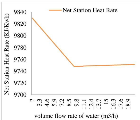
Fig. 11: Effect of variation of volume flow rate of water on heat rate of gas turbine
