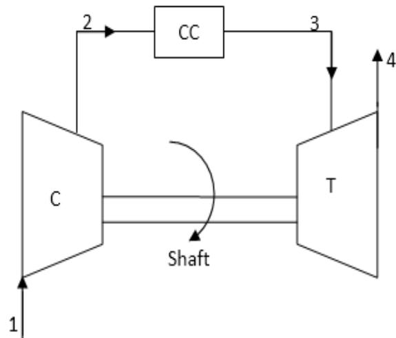
**Fig. 1:** Schematic diagram of the gas turbine unit
