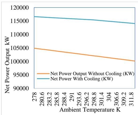
Fig. 6: Effect of ambient temperature on net power output
