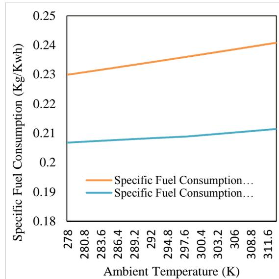
Fig. 7: Effect of ambient temperature on specific fuel consumption
