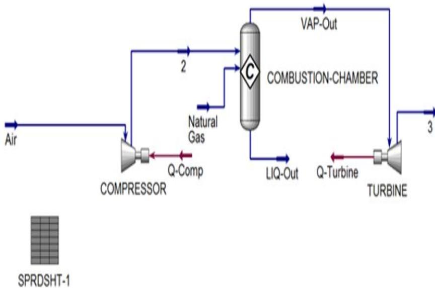
Fig 2: Flow chart of simulated simple gas turbine unit
