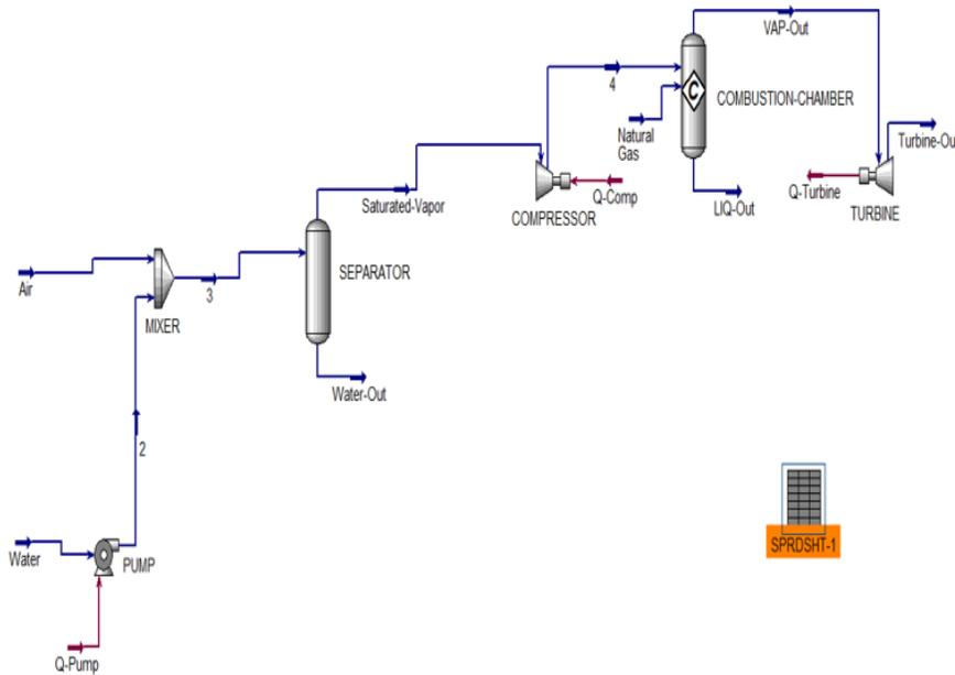
Fig. 3: Process Flow sheet for Gas Turbine with Fogging Unit
