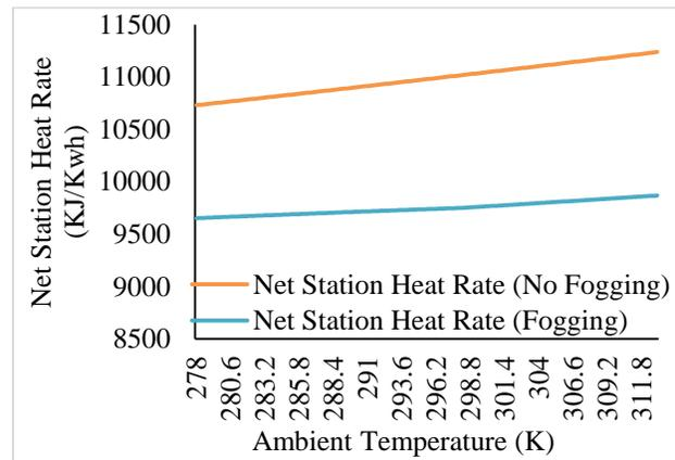
**Fig 4:** Effect of ambient temperature on heat rate
