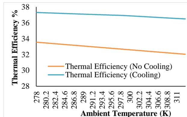
**Fig. 5:** Evaluation of the effect of ambient temperature on thermal efficiency of gas turbine plant
