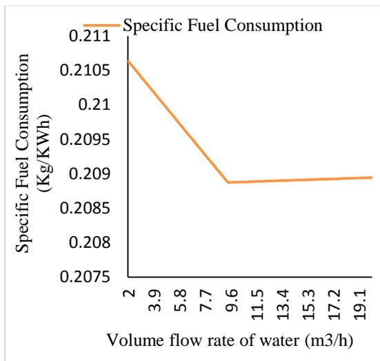
Fig. 10: Effect of variation of volume flow rate of water on specific fuel consumption of gas turbine
