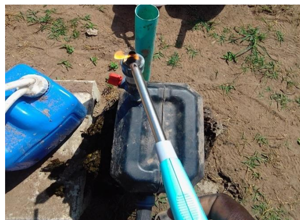
Fig. 9: Testing the flammability of produced biogas
