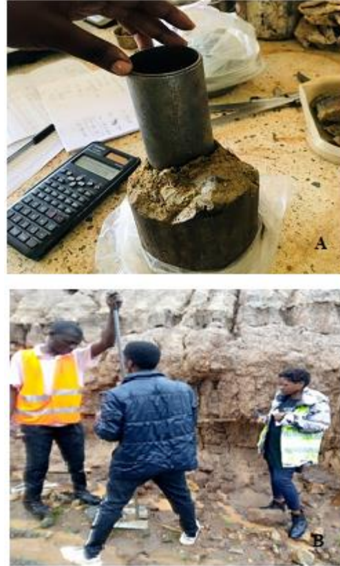
Fig. 2: Field and Laboratory Soil Tests (a) Laboratory Triaxial Soil Test; (b) Field Dynamic Probing Test
