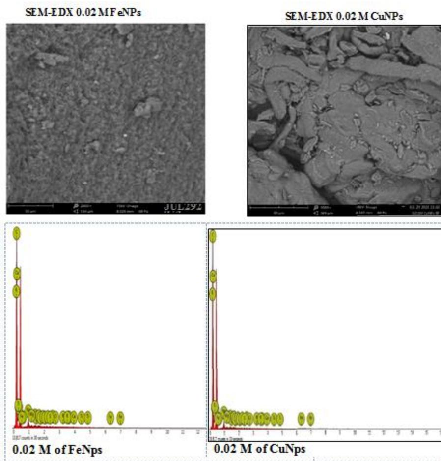
Fig 2: SEM Results of the Synthesized Iron and Copper Nanoparticles
