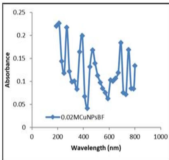
Fig 4: UV-Visible Spectrum CuNPs at 0.02M
