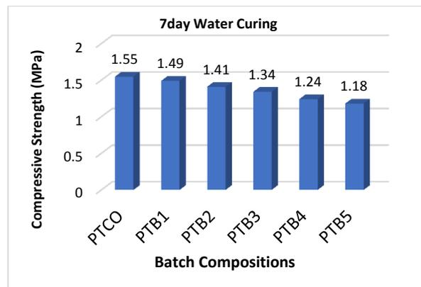
**Fig 3:** Compressive Strength of the Probe Test Bricks in 7-day of water Curing
