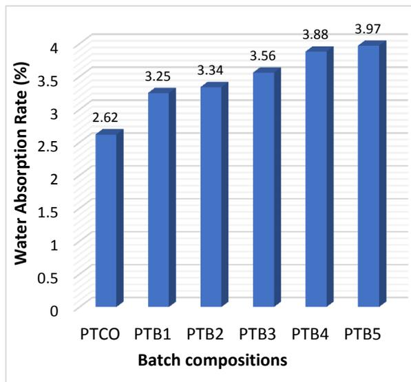
**Fig 2:** Water Absorption Rate of the Probe Test Bricks
