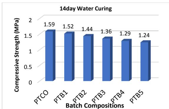
Fig 4: Compressive Strength of the Probe Test Bricks in 14-day of water Curing
