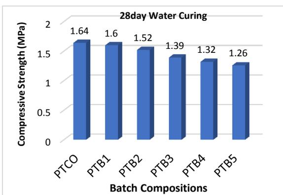
Fig 5: Compressive Strength of the Probe Test Bricks in 28-day of water Curing
