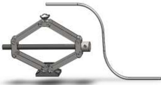
Fig. 2: Conceptual design 1 of a scissors jack
