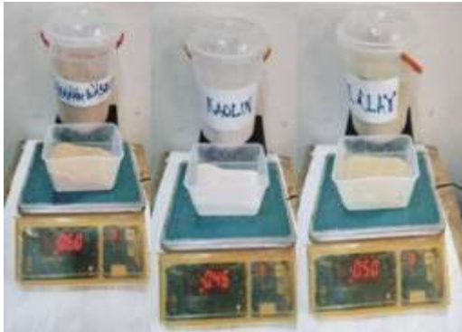
Plate 8: Measurement of samples for batch Compositions With Electronic Scale Model BL 20001
