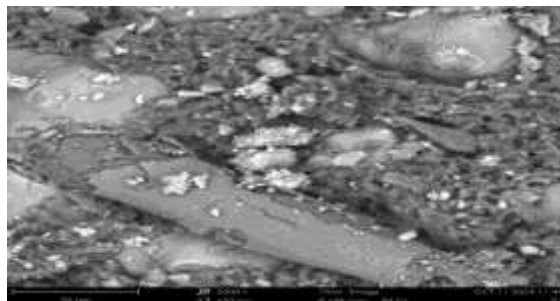
Plate 8: SEM image of BMOD after biosorption of Cr (VI) ion, 30µm
