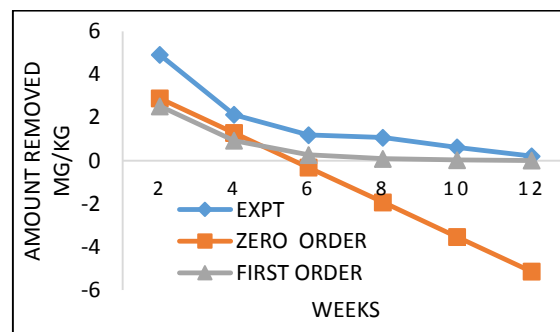
Fig 20. Kinetic plots for removal of Pyrene by cow dung during the remediation period.
