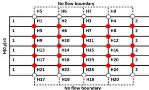
Fig 4: Schematic Diagram for Example 2
