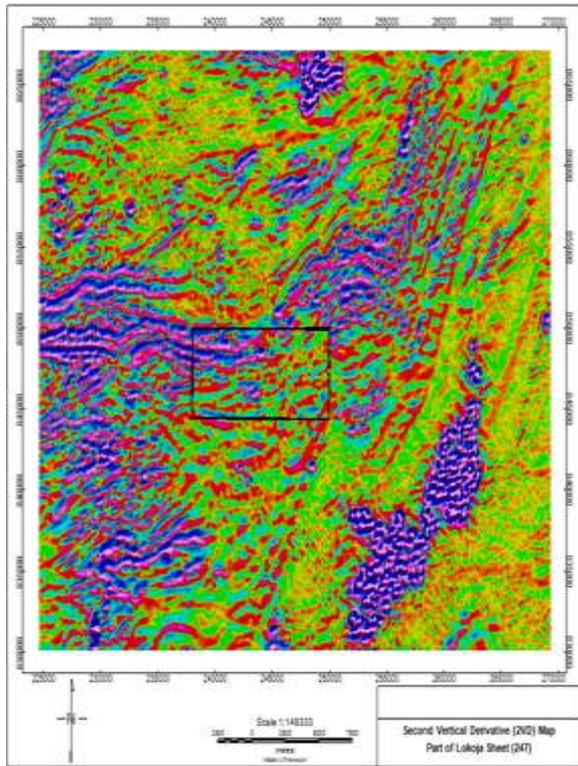
Fig 6: Second vertical derivative image of the tenement area shows near surface structures.
