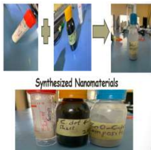
Fig. 3: Process flow diagram for the synthesis of ZnO-C.dot from groundnut shell
