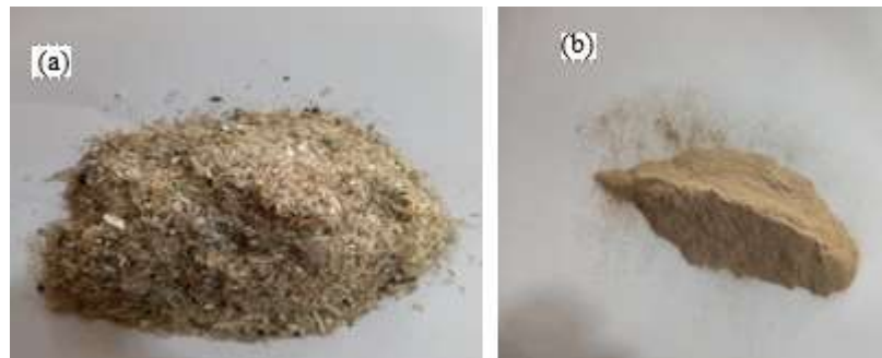
Fig 2: Processing of plastic powder (a) Ground plastic powder before sieving (b) Ground plastic powder after sieving
