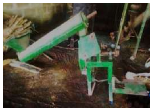
Fig 1: Fabricated oil palm nut cracking machine and conveyor
