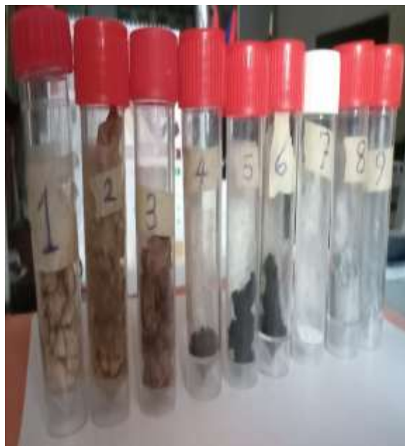
Figure 1: The synthesized zeolites using three agricultural waste materials and three methods of synthesis; from 1-9: MZSB, MZGS, MZCC, HZSB, HZCC, HZGS, FZSB, FZCC and FZGS
