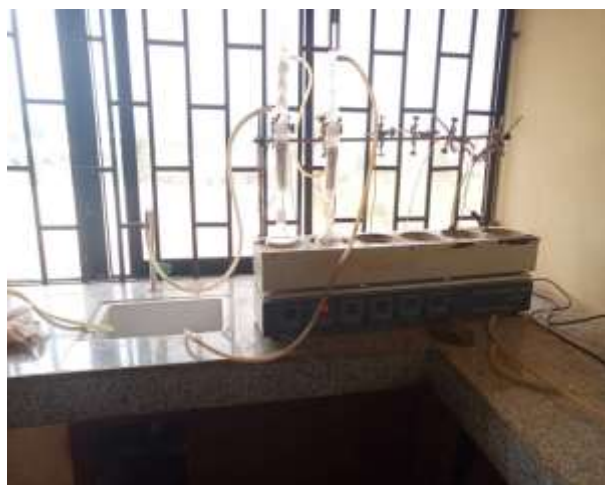
Plates 2: Complete set up of Soxhlet Extractor
