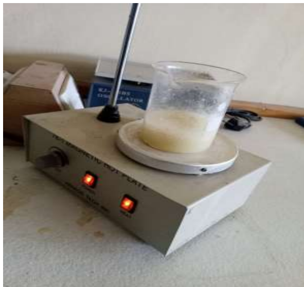
Plates 3: Stirring of the green synthesized titanium dioxide nanoparticle
