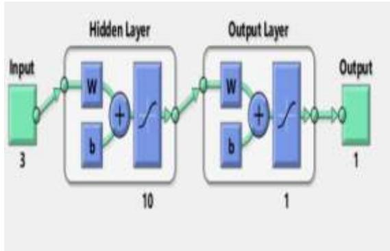
Fig 1: ANN architecture for Tool wear
