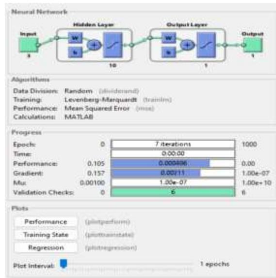
Fig 3: Network training diagram for predicting tool wear
