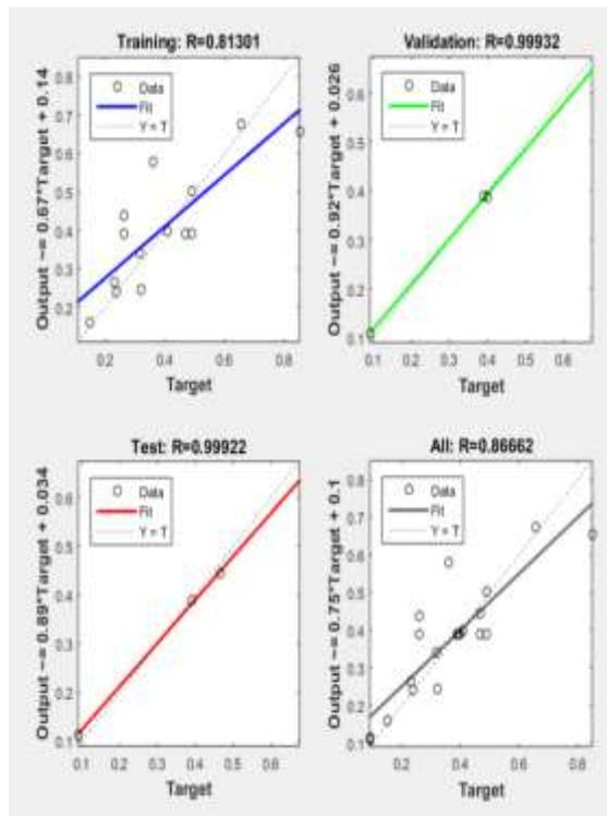
**Fig 6:** Regression plot of training, validation and testing for tool wear
