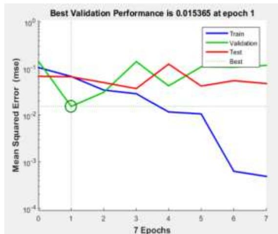
Fig 4: Performance curve for trained network to predict tool wear
